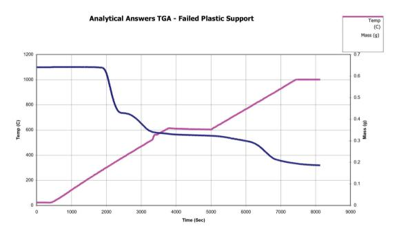
Temperature and mass as a function of time show instabilities in the material at elevated, constant temperatures, as well as a simple verification of correct operation of the balance and furnace over the course of the run.
